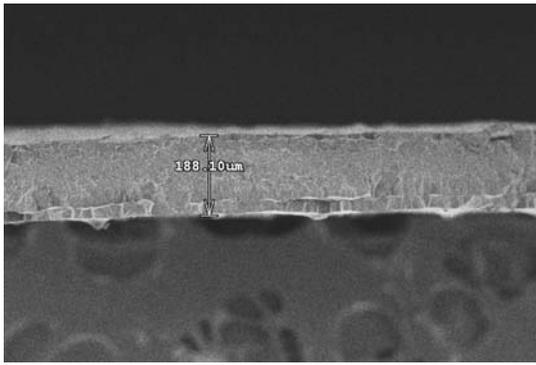
**Fig. 2** Scanning electron micrographs of PES film thickness
